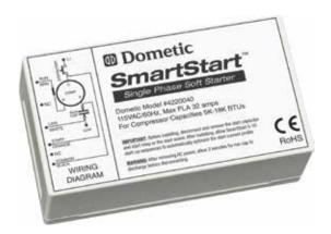
The SmartStart™ is a unique device that smooths out startup power demand of the boat air conditioner's compressor instead of spiking it, reducing amp requirements by up to 65%. The technology uses dynamic feedback control to reduce the inrush of current by starting the compressor motor slowly. No other soft starter in the industry provides better performance.
